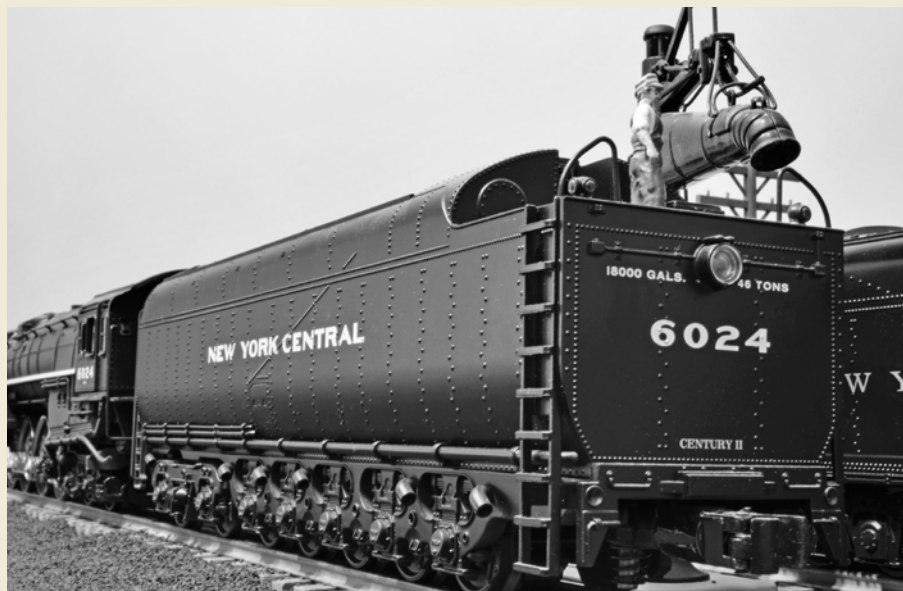
▲ The fireman prepares to swing the waterspout over the open hatch to fill the huge PT-5 tender, which holds 18,000 gallons of water and 46 tons of coal. This enormous capacity enables the engine to make the 900-mile run from New York to Chicago with just one coaling stop.
