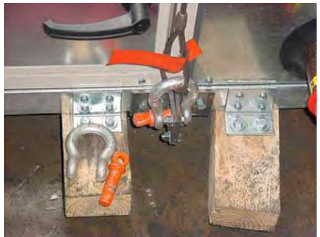
FIG. 1-5 – PROPER LIFTING WITH SHACKLE AT LIFTING LUG
