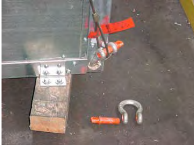
FIG. 1-4 – PROPER LIFTING WITH SHACKLE AT CORNER
