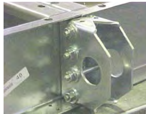
Baserail Lifting Lugs Assembled
