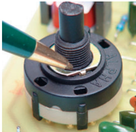
To set switch S1 for eight positions, turn its rotor fully anticlockwise and then make sure that the stop pin is in the slot between the moulded '8' and '9' figures.
