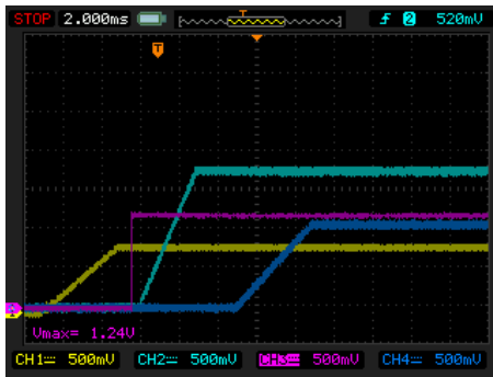
Yellow – VCCPSINT_LP Pink – PSPLL Light Blue – VCCPSAUX Dark Blue – VCCO PSDDR 1.1V
