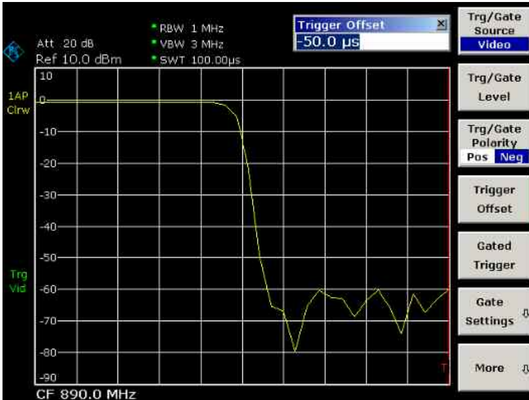
Fig. 5–11 Falling edge of the GSM burst displayed with high time resolution
