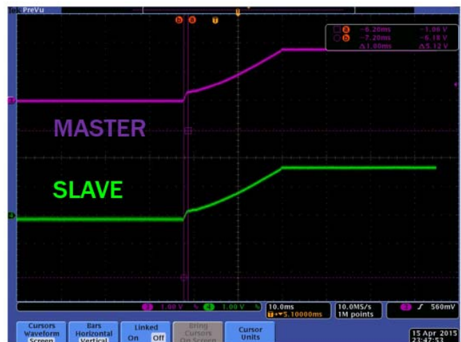
FIGURE 3. ISL8002B TRACKING START-UP
