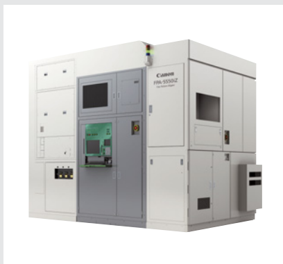
The FPA-5550iZ is an i-line stepper employing the FPA-5500 platform with proven high performance and reliability, which enables high throughput such as short exposure time through a high-acceleration wafer stage.
