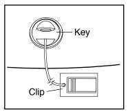
a moment, the displays will light. **IMPORTANT: In an** emergency, the key can be pulled from the console, causing the walking belt to slow to a stop. Test the clip by carefully taking a few steps backward; if the key is not pulled from the console, adjust the position of the clip.
