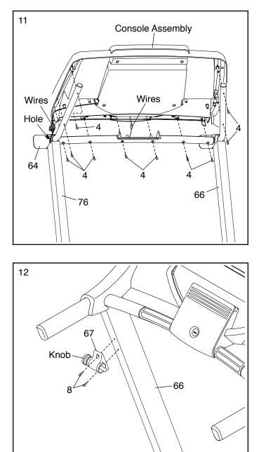
12. Attach the Latch Pin Assembly (67) to the Left Upright (66) with two #10 x 3/4" Screws (8); start both Screws, and then tighten them. Orient the Latch Pin Assembly so that the knob is on the indicated side.
