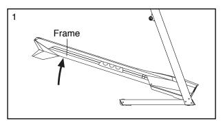
2. Hold the frame firmly with your right hand. Pull the latch knob to the left and hold it. Raise the frame until the hole in the platform cushion is aligned with the latch pin. Then, slowly release the latch knob; make sure that the latch pin is fully inserted into the platform cushion.
