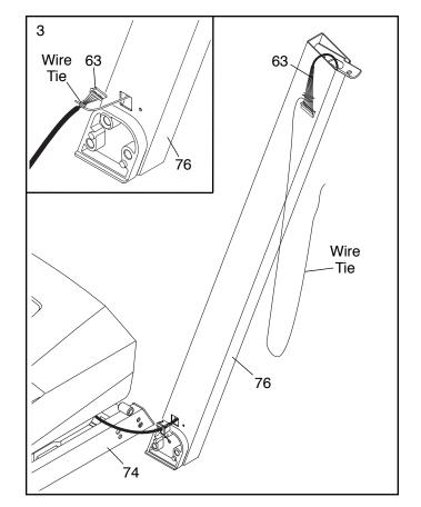
Lay the Right Upright (76) near the Base (74) as shown. Attach the ground wire to the Base with a #8 x 1/2" Ground Screw (1).
