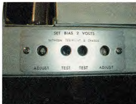
Photo 3: The grid bias adjustment test points/potentiometers.
