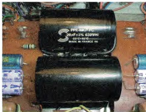
Photo 4: The replacement polyester-film HT smoothing electrolytics.
