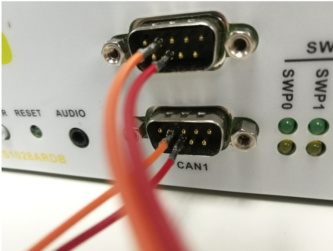
Figure 45. Physical connection for CAN using LS1028ARDB
