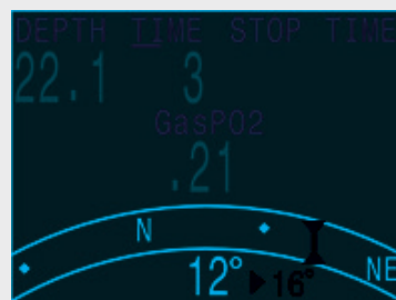
The offset between current and marked heading is now shown (in this example 16°)
