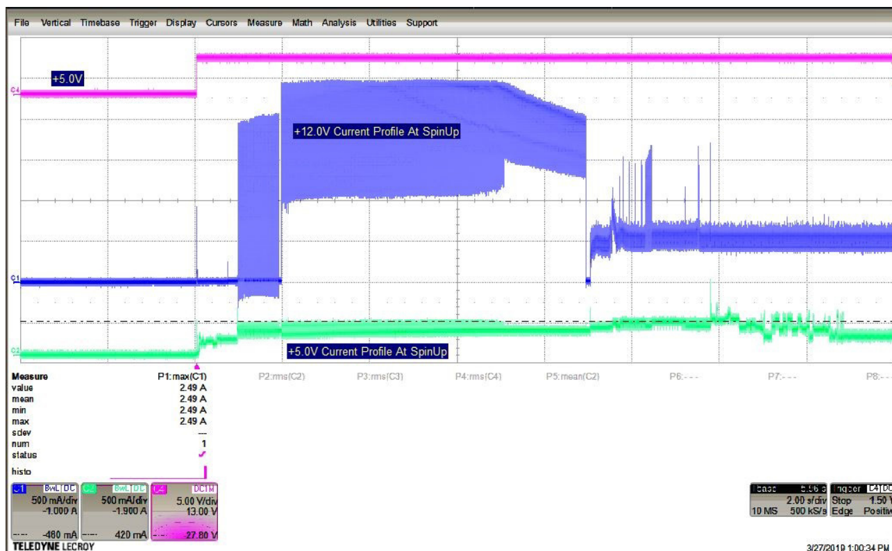
Figure 1. 8TB model current profiles.
