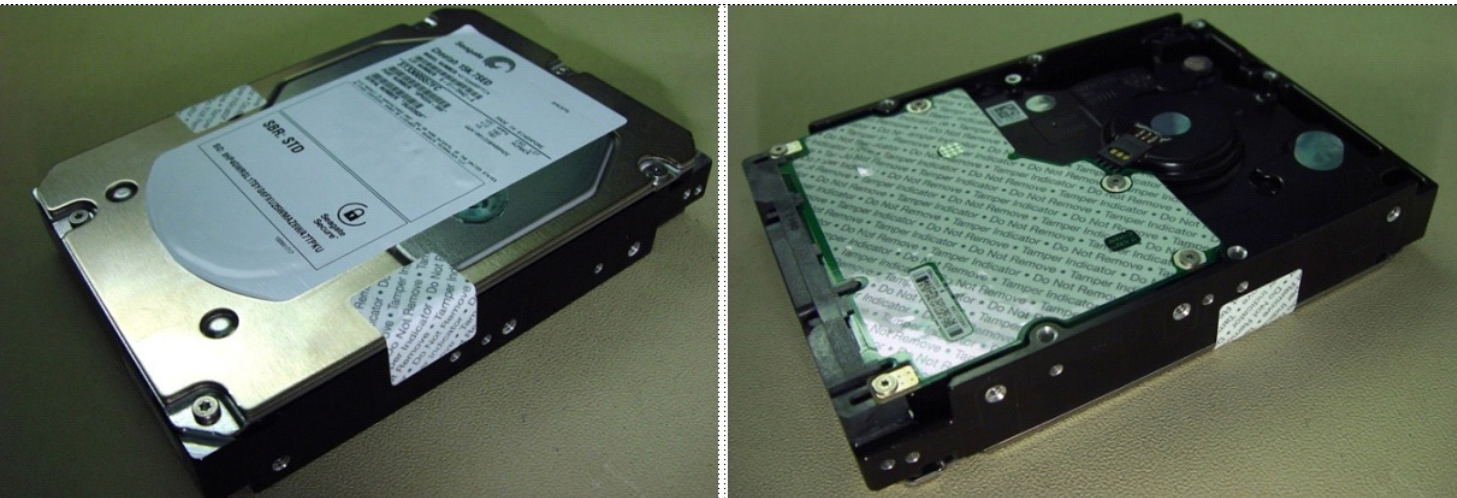
Figure 11. Example of FIPS tamper evidence labels.
