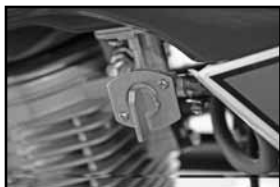
Fuel Valve ON
