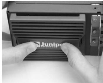
Figure 30: Securing the Filter Cover
