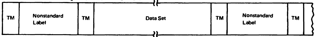
Example 3 -- Tapemarks Delimiting the Labels and the Data Set
