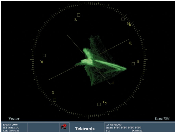
Figure 6. The graticule is the part colored gold and the trace is colored green. The colors of the graticule and trace are user selectable. These are the defaults. Many colorists prefer to use white or gray only to keep their eyes from being affected by the saturation of the colors.
