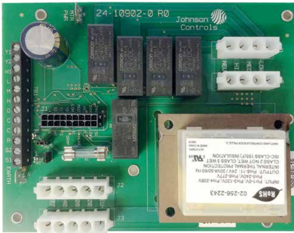
Figure F.1: Fan Relay Board (FRBii)
