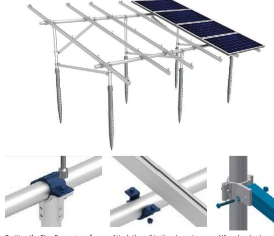
Position the Pipe Cap on top of the vertical pipe and lay the horizontal pipe into the Pipe Cap assembly. Attach the rail to the pipe using the aluminum pipe clamp kit. To prevent galvanic reaction, the PVC insulator must be installed be-tween the steel pipe and the aluminum rail.
