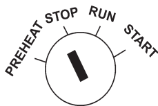
Figure 71. Ignition Key Switch (STOP position)
