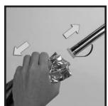
5 Grasp both the packing bag and roller firmly and pull them off the long roller waxer handle. To do this, push the roller away from the handle grip toward the bar to compress the retaining spring. This will allow you to slide the roller over the end cap. Seal bag tightly to prevent premature drying. Store in the provided packing tube and put in a safe place away from children and pets until next use. ➤
