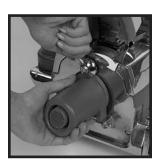
When using the blower attachments, the Air Intake Guard must be attached to the front of the unit.
