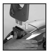
Remove the cord from the handle. With the Upright Handle ① in the vertical position, push the Handle Release Button ④, located at the base of the handle, and pull the handle straight up and out of the slot. (Bag not shown for clarity.)
