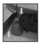
Press the Toe-Touch Control Upper Pedal ® to lower the brush one notch at a time. Lower the brush as far as the Toe-Touch Control will allow.
