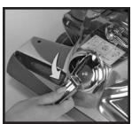
2 Flip out the handle on the Belt Lifter ②. Use it to turn the Belt Lifter fully to the left (counter-clockwise) until it stops and the red arrows line up. This stretches the belt and lifts it off the motor shaft. Return the handle on the Belt Lifter to its closed position.
