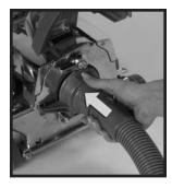
At the connector end of the Attachment Hose, you will notice two hooks. Place the hooks over the ends of the Attaching Bar ②, then push the opening of the hose up against the *Sentria*® system.
