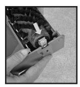
Align the metal ends of the brush with the slots on the tray and push the brush in until it snaps into place. The brush will only fit the tray the correct way.
