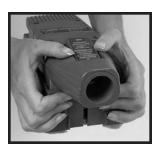
5 With the Turbo Accessory on a level surface, wrap the Sander Dust Shroud around the Sander with the opening to the rear and snap it closed. ➤
