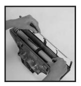
Pull on the rear edge of the Rug Plate to remove from the nozzle. Note the Brush Roll Bristle Height Adjustment setting (1, 2, or 3). Lift out the belt and Brush Roll. ➤
