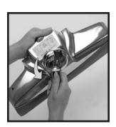
Using the handle on the Belt Lifter (20), turn it to the left (counterclockwise) until the red arrows line up. This will stretch the belt in preparation for returning the nozzle to the *Sentria* system.
