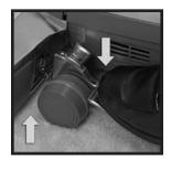
To turn your *Sentria*<sup>®</sup> system OFF, press the Toe-Touch Control Bottom Pedal <sup>®</sup> all the way down until nozzle is fully raised.
