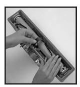
Make sure the Brush Roll Bristle Height Adjustment setting (1, 2, or 3) is the same on both ends as when the brush was removed. See below for discussion of the Brush Roll Bristle Height Adjustment (1, 2, or 3). Place the belt and Brush Roll back into the nozzle. One of the plastic Brush Roll ends is larger than the other, thus the Brush Roll will only fit in the nozzle one way.
