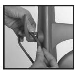
With the Upper Cord Hook in the up or 12 o'clock position, route the cord toward the rear of the unit and slide the cord in to the c-shaped holder on the Upper Cord Hook. The cord can now be wrapped around the Upper and Lower Cord Hooks for storage. To quick-release the cord for use, rotate the Upper Cord Hook down to the 6 o'clock position. The c-shaped holder is designed to hold the cord securely in place and prevent the first loop from dropping to the floor.
