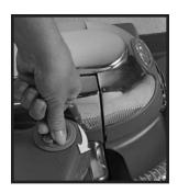
Turn the Suds Control Valve all the way to the right (clockwise) to the ON position. Turn the *Sentria* system ON and engage Tech Drive<sup>®</sup> power assist (see page 7 for details). Suds flow will begin immediately.
