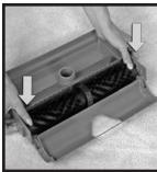
Push down carefully on the ends of the brush with your thumbs. The brush will snap out and the belt can be replaced.
