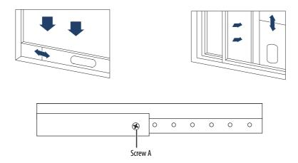
4 Insert the hose adapter into the vent panel, then slide the adapter until it clicks into place.
