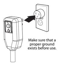
To prevent damage to the adapter's ground terminal, hold the adapter in place while plugging or unplugging the air conditioner.
