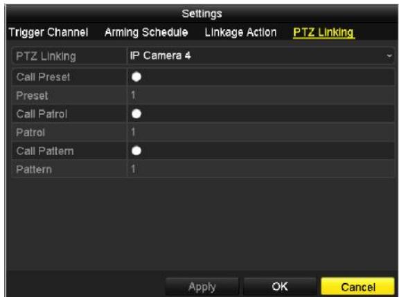
Figure 8. 7 Set PTZ Linking of Alarm Input
