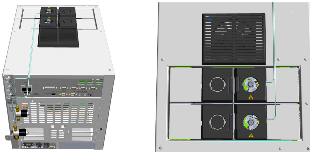
Figure 111. Front and Back PTV Cryo System with Carbon Dioxide
