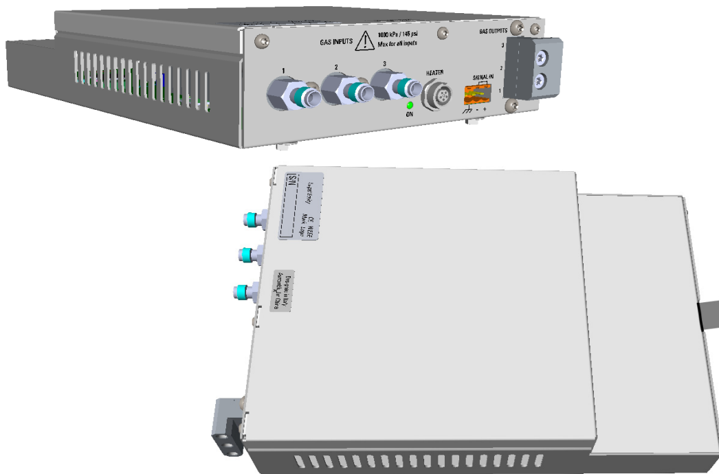
Figure 165. GDI Electrical Interface
