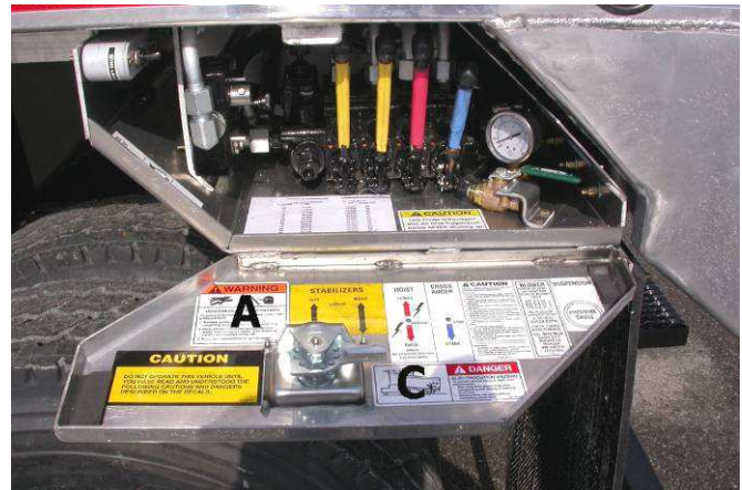
Fig. 3-4 Control Box Trailer (Typ)
