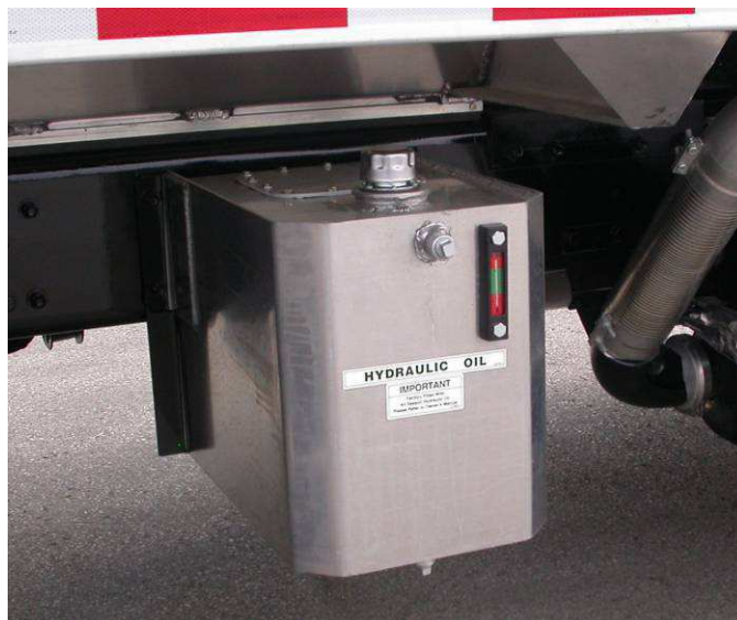
Fig. 7-6 Hydraulic Tank (Typical)
