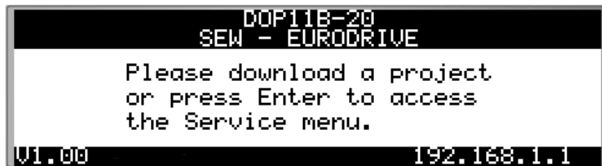
Figure 17: DOP11B-20 initial screen in delivery state
