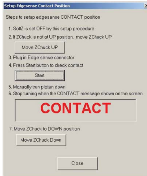
Figure 808: CM500 Prober Setup Edgesense Contact Position window
