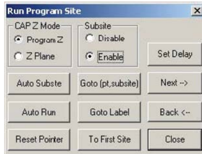
Figure 820: CM500 Prober Enable Subsite
