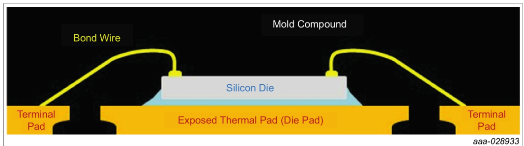
Figure 4. Cross-section of a sawn QFN with exposed pad
