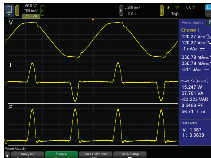
PA2201A making an efficiency measurement on signal containing both AC and DC
