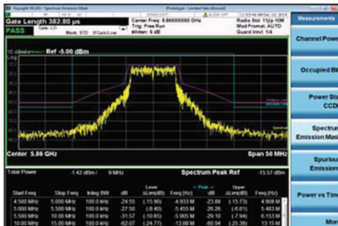
SEM measurement on a 10-MHz FCC Class A, 802.11p transmitter with 0-dBm maximum output power by the Keysight N9077 WLAN measurement application
