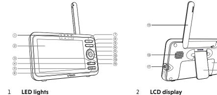
Indicate the different statuses of the parent unit. For details, refer to **Parent**
