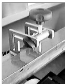
Jacking screw against bedknife (Bar shown rotated to vertical position for clarity)
