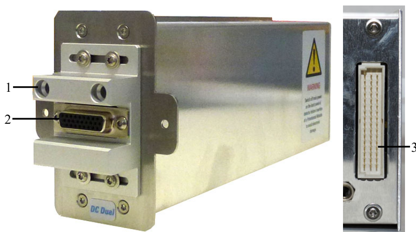
Fig. 6: Side and rear view of a potentiostat module for DC Mode
