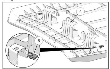
3. If vehicle is equipped with windshield: Install seal ⑤ onto ridge of roof panel ④.
