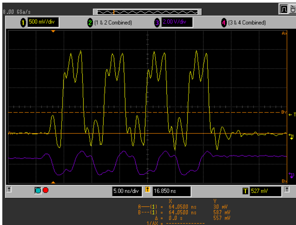
Figure 5. Scope Capture of Filtered DQS0 Signal
