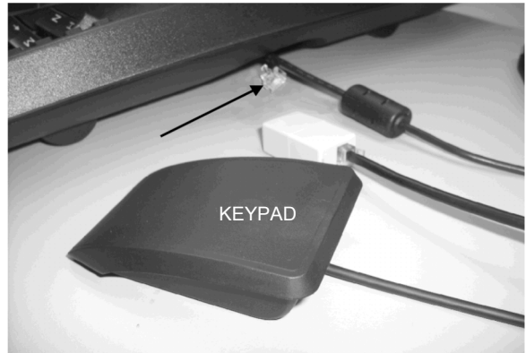
Figure 1. Single pedal, FS007RJ11 showing plug from keyboard.
