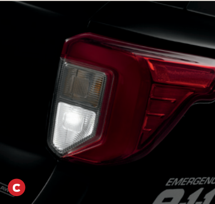
Taillamp Lighting Solution. Includes halogen base lamps and (2) integrated hemispheric lighthouse white LED marker lights.
