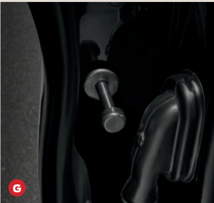
Hidden door lock plungers. Manual lock rod with inoperable rear door handles.
