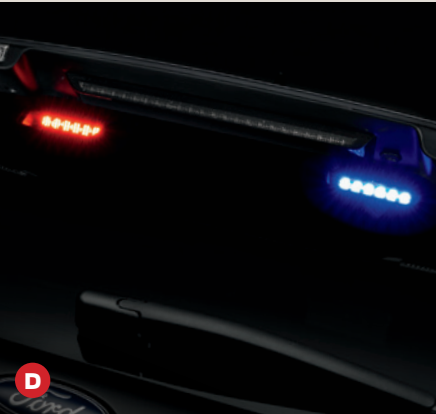
Rear Lighting Solution. Includes (2) backlit flashing, linear high-intensity LED lights (driver side red; passenger side blue) with surround cover mounted inside the liftgate glass and (2) backlit flashing, linear high-intensity LED lights mounted inside the liftgate lip.
