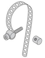
Mounting on round cylinders; cylinder diameter 80...200 mm material: Metal A2 1.4301 (AISI 304); two tie bolts (material: Metal CuZn, alternatively metal A2 1.4301 / AISI 304) cylinder screw M3 x 20; (DIN 912-A20)
