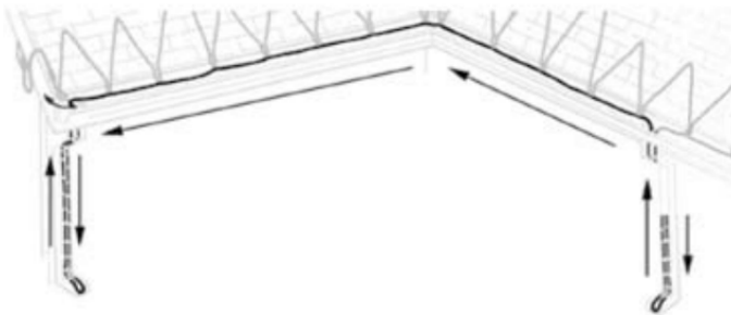
Figure 8. Cable routed back along the roofline in the gutter and Downspouts
