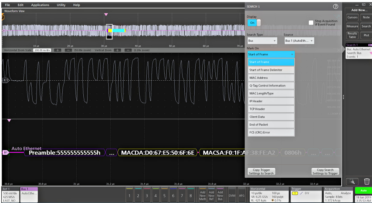
Searching on a specific data pattern on the Automotive Ethernet (100BASE-T1) bus and automatically searching on Start of Frame.
