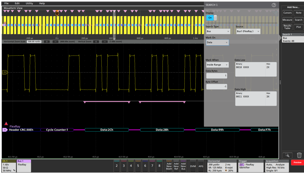
Decoded FlexRay bus, with all data values in a specific range marked with pink brackets.
