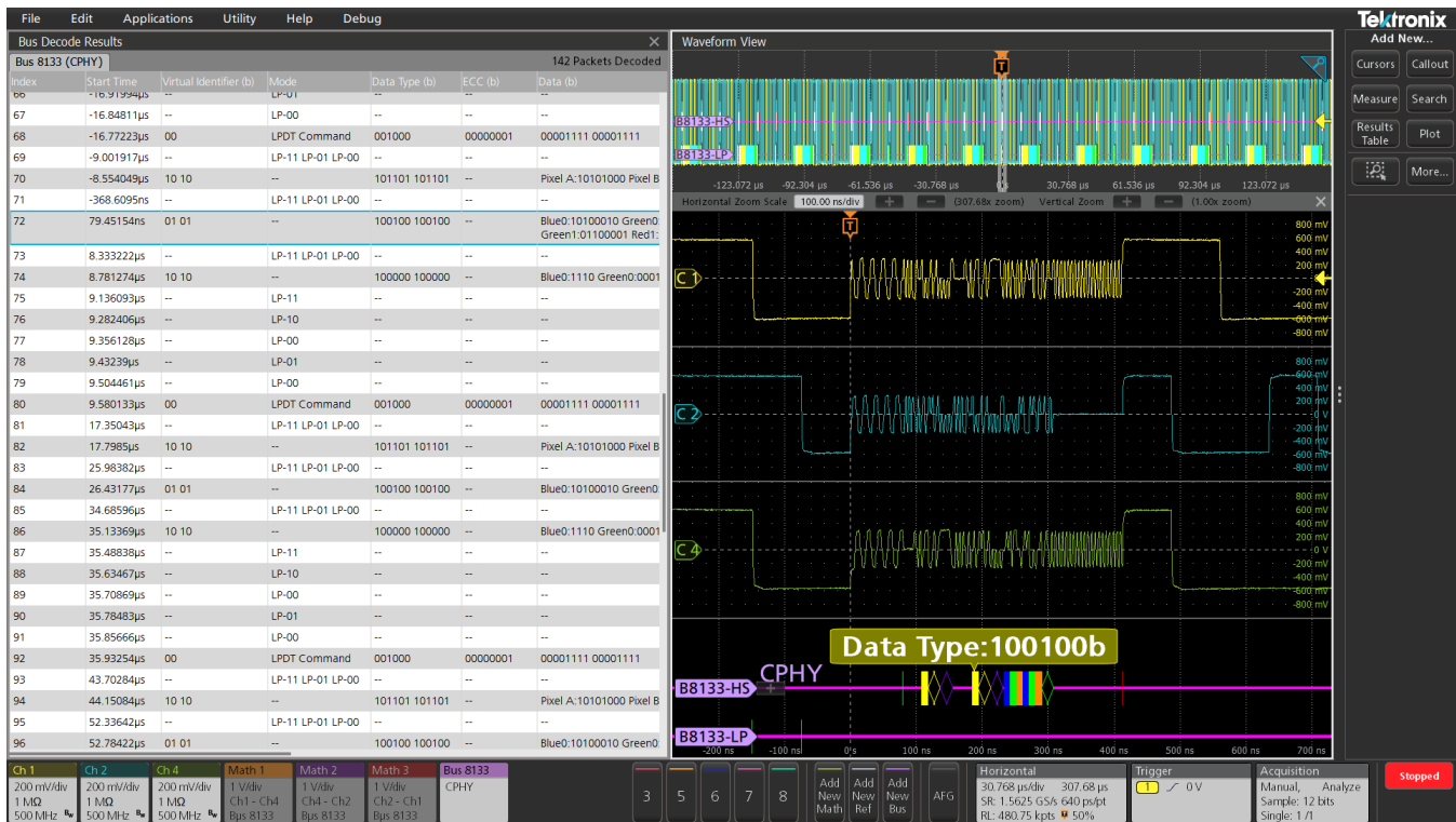
The protocol decode results table provides a time-stamped, tabular view of all captured pixel packets on the CPHY bus
