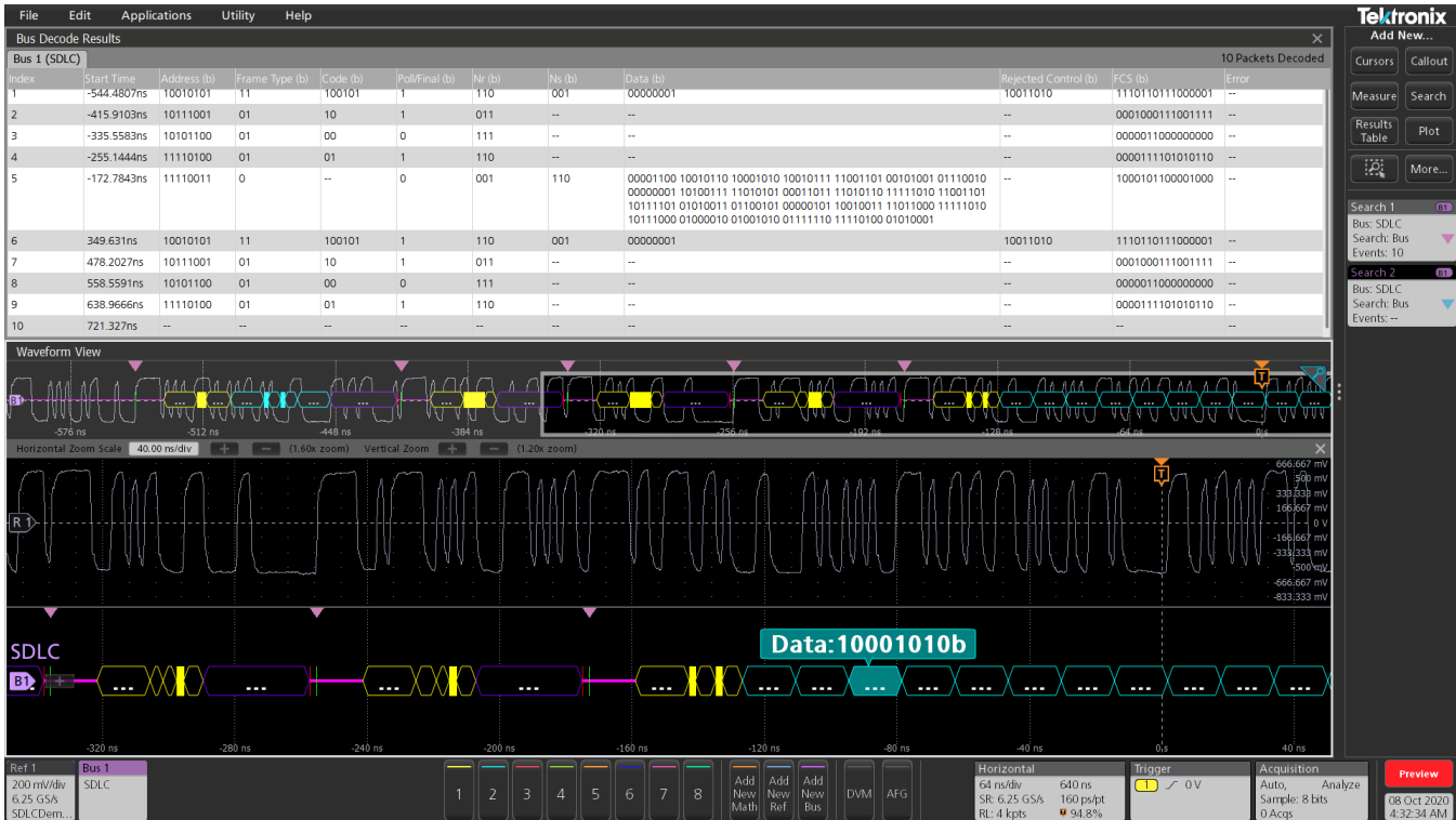
The Protocol Decode Results Table provides a time-stamped, tabular view of all captured packets on the SDLC bus.
