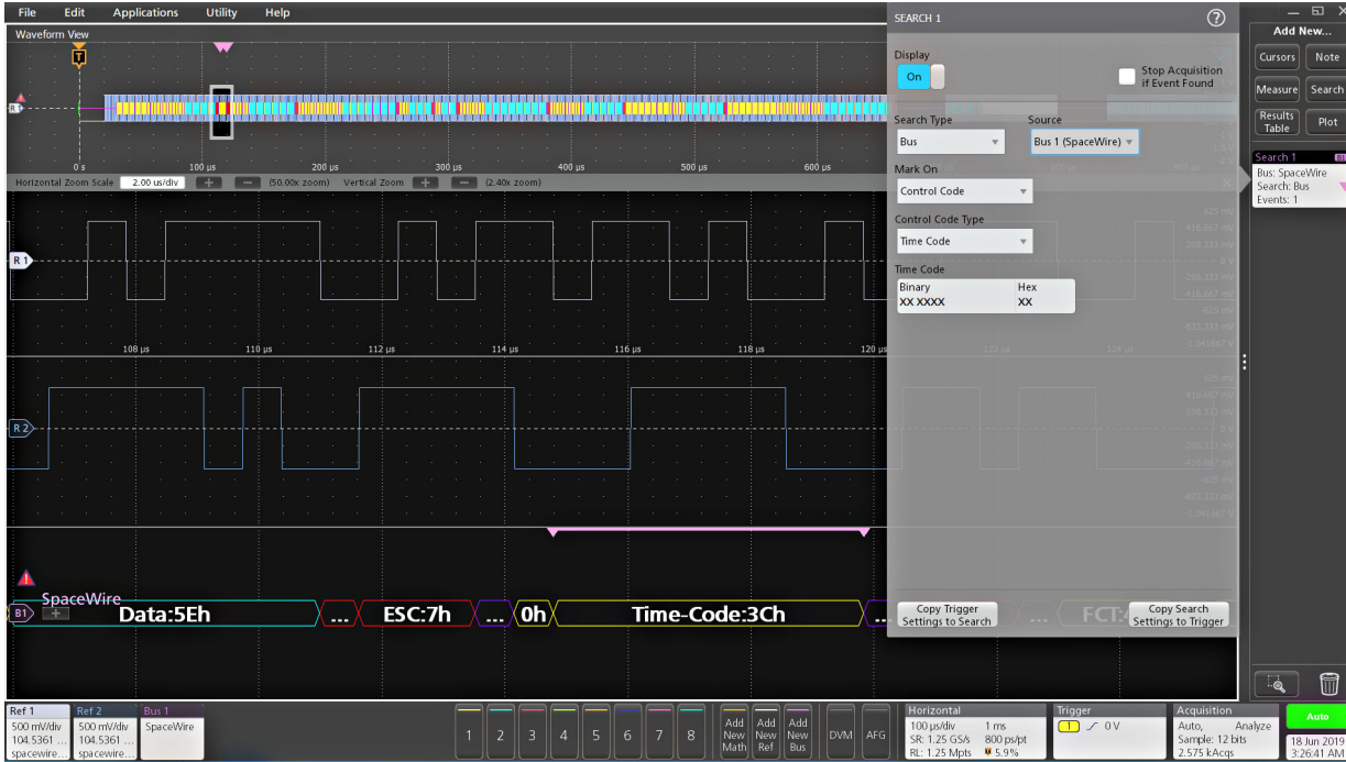
Searching on a specific data pattern on the SpaceWire bus and automatically searching on Sync.
