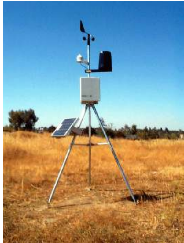
110-WS-16 Modular Weather Station with NEMA-4X Enclosure & Solar Panel
