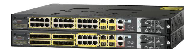
**IE3100:** 1 RU, fixed, hardened switch with REP support; 2 x GE & up to 24 FE ports (copper) or 16 FE SFP and 8 FE (with PoE), swappable flash memory.
