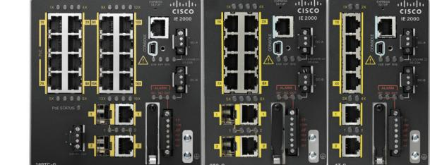
**IE2000:** Compact, secure, fixed hardened Layer 2 access DIN-rail mounted switch with REP, IEEE 1588, Ethernet/IP, PROFINET support; 2 x GE & 4, 8, or 16 x FE ports, swappable flash memory, NAT PoE and conformal coating available.
