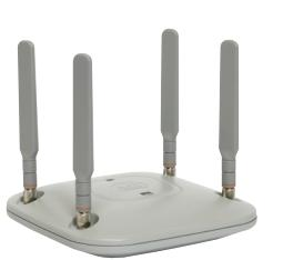
**Allen Bradley Stratix 5100™ Wireless Access Point (AP):** 802.11n Wi-Fi autonomous access point. 3x4 MIMO technology with three spatial streams. External antennas. Integrated Common Industrial Protocol (CIP) stack.
