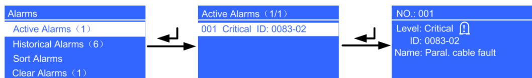
Figure 4-12 Active Alarms screen
