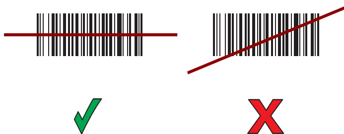
Figure 11 Linear Scanner Aiming Pattern
