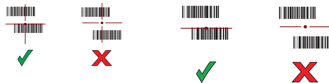
Figure 9 Pick List Mode with Multiple Barcodes in Aiming Pattern: Standard and Extended Range
