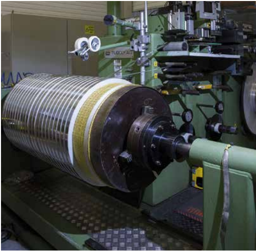
HV winding with strip technology
