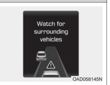
If the vehicle ahead (vehicle speed: less than 30 km/h (20 mph)) moves to the next lane, the warning chime will sound and a message "Watch for surrounding vehicles" will appear. Adjust your vehicle speed for vehicles or objects that can suddenly appear in front of you by depressing the brake pedal.
