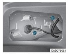
Loosen the assembly retaining nuts.
