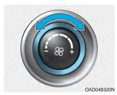
The fan speed can be set to the desired speed by turning the fan speed control knob.
