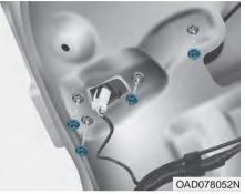
Disconnect the connector and then remove the nuts by turning the nuts counter clockwise.
