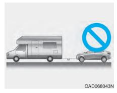
Your vehicle is not designed to be dinghy towed (with 4 wheels on the ground) behind a motor home. To avoid serious damage to your vehicle, do not tow your vehicle with four wheels on the ground.
