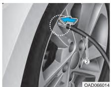
3. Unscrew the valve cap from the valve of the flat tire and screw the filling hose (2) of the sealant bottle onto the valve.
