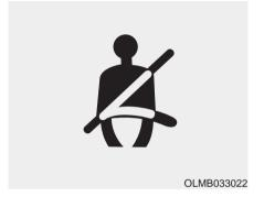
As a reminder to the driver, the seat belt warning light will illuminate and warning chime will sound for approximately 6 seconds each time you turn the ignition switch ON if the seat belt is unfastened.
