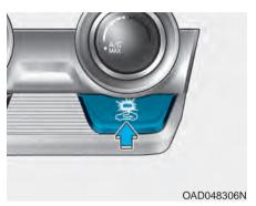
This button is used to select the outside (fresh) air position or recirculated air position.
