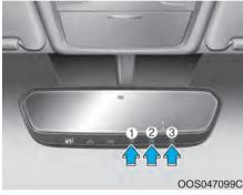
Press and release the programed HomeLink button to activate the garage door. 4. Once the garage door is stopped, press and release the "Learn" or "Smart" button on the Garage door opener within 1 minute from the time of pressing the programed HomeLink button on mirror.
