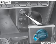
The power outlet is designed to provide power for mobile telephones or other devices designed to operate with vehicle electrical systems.
