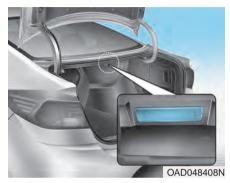
The trunk room lamp comes on when the trunk is opened.
