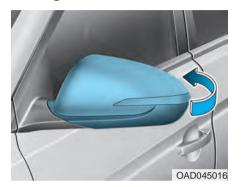
To fold the side view mirrors, grasp the housing of the mirror and then fold it toward the rear of the vehicle.
