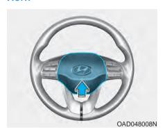
To sound the horn, press the area indicated by the horn symbol on your steering wheel (see illustration). The horn will operate only when this area is pressed.
