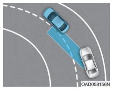
The system may not operate properly when driving on a curved road. In certain instances, the system may recognize a vehicle in the same lane.
