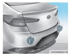
The rear radars are located inside the rear bumper for detecting the side and rear areas. Always keep the rear bumper clean for proper operation of the system.
