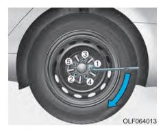
13. Use the wheel lug nut wrench to tighten the lug nuts in the order shown. Double-check each lug nut until they are tight. After changing tires, have an authorized HYUNDAI dealer tighten the lug nuts to their proper torque as soon as possible. The wheel lug nut should be tightened to 11~13 kqf-m (79~94 lbf-ft).
