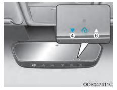
5. If the both indicator (4) and (6) are flashing rapidly for about 5 seconds, the two way synchronization is completed.
