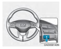
When the Smart Cruise Control system is ON, you can set and maintain the distance from the vehicle ahead of you without pressing the accelerator or brake pedal.
