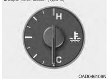
This gauge indicates the temperature of the engine coolant when the ignition switch or Engine Start/Stop button is ON.
