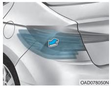
Remove the rear combination light assembly from the body of the vehicle.
