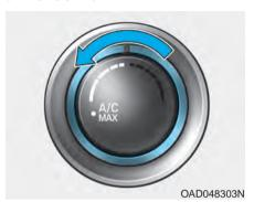
The MAX A/C mode is used to cool the inside of the vehicle faster. Air flow is directed toward the upper body and face.
