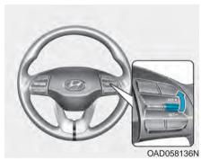
Push the toggle switch up (RES+). If the vehicle speed is over 30 km/h (20 mph), the vehicle will resume the preset speed.
