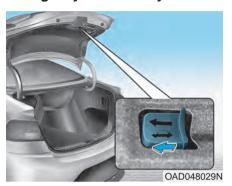
Your vehicle is equipped with an Emergency Trunk Safety Release lever located inside the trunk. When someone is inadvertently locked in the trunk, the trunk can be opened by moving the lever in the direction of the arrow and pushing the trunk open.
