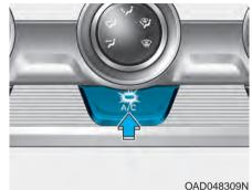
Press the A/C button to turn the system on (indicator light will illuminate) and off.
