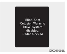
Blind-Spot Collision Warning (BCW) system disabled. Radar blocked
