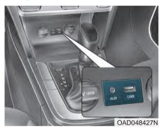
You can use an AUX port or USB cable to connect audio devices to the vehicle AUX or USB port.
