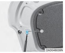
4. Pull out the support rod and prop the hood open with the support rod (3).
