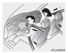
Your vehicle is equipped with driver's and front passenger's Pre-tensioner Seat Belts (Retractor Pretensioner and Emergency Fastening Device System). The purpose of the pre-tensioner is to make sure the seat belts fit tightly against the occupant's body in certain frontal collisions. The Emergency Fastening Device System may be activated in certain crashes where the frontal collision is severe enough, together with the air bags.
