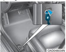
The fuel filler door must be opened from inside the vehicle by pulling up the fuel filler door release lever.
