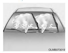
Contamination of either the windshield or the wiper blades with foreign matter can reduce the effectiveness of the windshield wiper functionality. Common sources of contamination are insects, tree sap, and hot wax treatments used by some commercial car washes. If the blades are not wiping properly, clean both the window and the blades with a clean cloth dampened with washer fluid.
