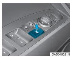
The driver can disable the power window switches on the rear passenger doors by pressing the power window lock switch.
