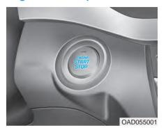
Whenever the front door is opened, the Engine Start/Stop button will illuminate and will go off 30 seconds after the door is closed.
