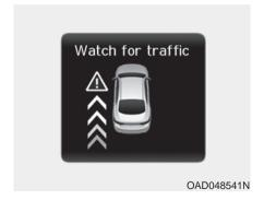
Once the system decides it is dangerous for a passenger to open a car door by sensing the approaching of a car from behind when the person is opening the door, the warning message "Watch for traffic" appears and the alarming sound will continue for five seconds
