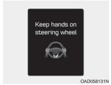
If the driver takes their hands off the steering wheel for several seconds while the LKA system is activated, the system will warn the driver.
