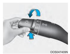
The High Beam Assist (HBA) is a system that automatically adjusts the headlamp range (switches between high beam and low beam) according to the brightness of other vehicles and road conditions.
