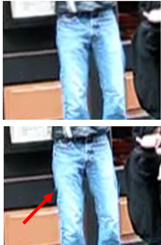
Figure 5: With local alignment (top) and without (bottom). Note that before the alignment the middle part of the person’s leg tears on the left edge of his jeans.
