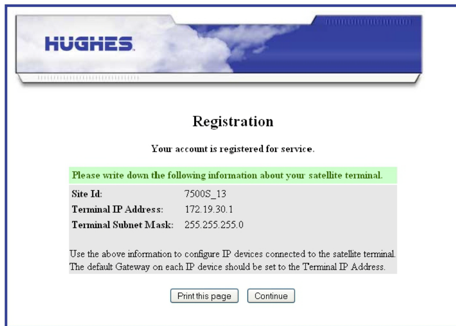
Figure 42: Registration screen with router identification information
