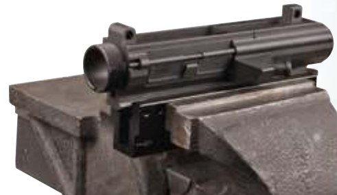
Use the Pic Rail of an AR Upper or other device to mount into your bench vise
