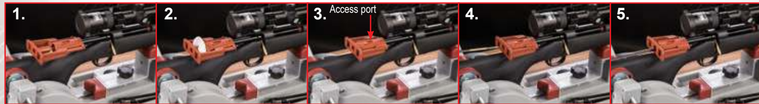
1. Insert the RAPID ™ and lock it in place 2. Pull out the sliding guide and insert a patch 3. Access port Push the sliding guide closed and add solvent to the access port soaking the patch 4. Insert a jag into the guide hole and push the patch down the barrel 5. Push the patch all the way through the barrel and repeat steps 1-4 until the barrel is clean
