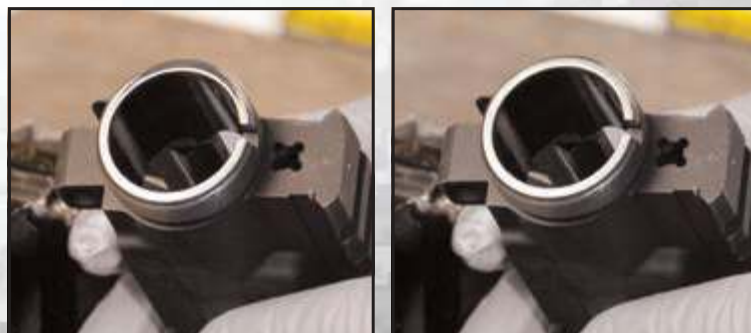
Showing a poor lapping job vs. a good lapping job.
