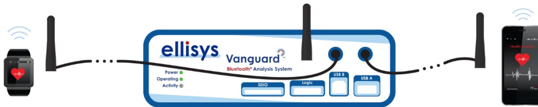
Figure 13 Bluetooth Capture Diversity - Externally Cabled
