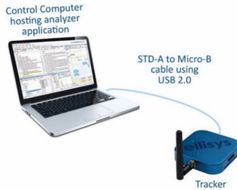
Figure 10 Basic Setup for Tracker (USB for Control and Power)
