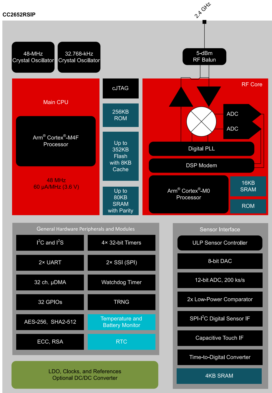
Figure 4-2. CC2652RSIP Hardware Overview
