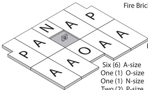
Figure 13a – Step 1, Bottom Firebrick Arrangement
